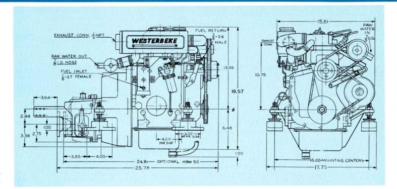
Westerbeke 10 two provides two cylinder, four cycle smoothness in a lightweight, compact engine. Cylinder head and block are cast iron for strength and long life, while aluminum is used in nonwearing parts for light weight. The performance from this 28 cubic inch space saving engine will amaze you!
